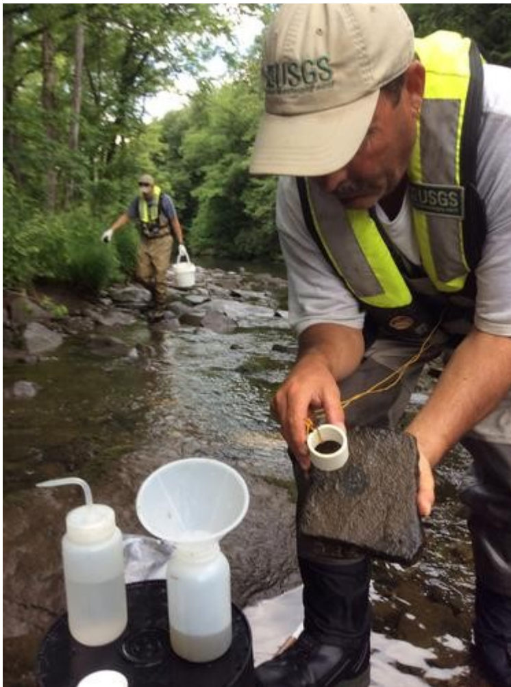
Figure 3-1. Geological Survey (USGS) scientist using a section of PVC pipe to collect standardized periphyton sample.
